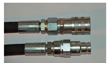
Above: 50 metre hydraulic umbilical (top first). 100 metre hydraulic umbilical (second). Hose end quick release fittings (third).
